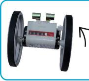
Measures the length in meters having a gear ratio 1:2. Also measures in meters and lengths having a gear ratio 5:1 with two knurled/rubber wheel ½ meter circumference. The counter is fitted on L bracket with a hinge for titling over when not in use
