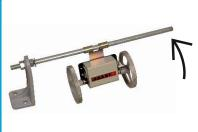
Measures the length in meters with two knurled/rubber wheels - 1/3 meter circumference. The counter is fitted on a bracket. This assembly is mounted, on L bracket with 12.7 mm (1/2") diameter 50 cm long rod. Stopper is provided to adjust pressure on the wheels.
